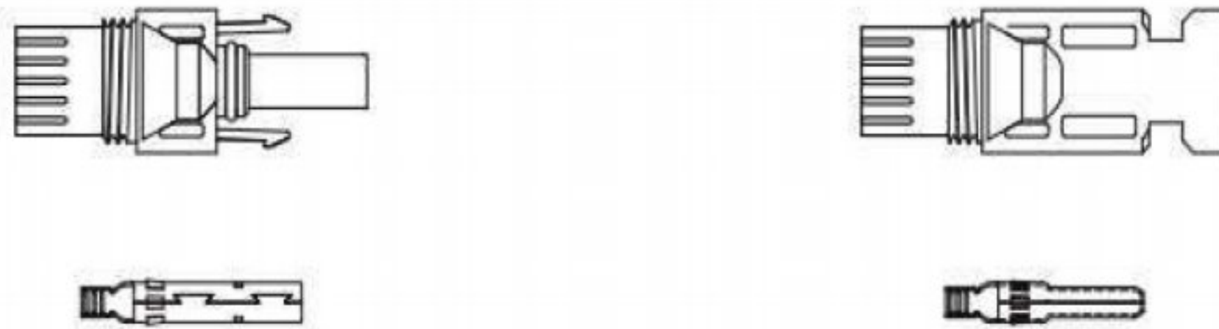
Figure 2.11 Photovoltaic input connector: DC+ connector left DC-Connector right
